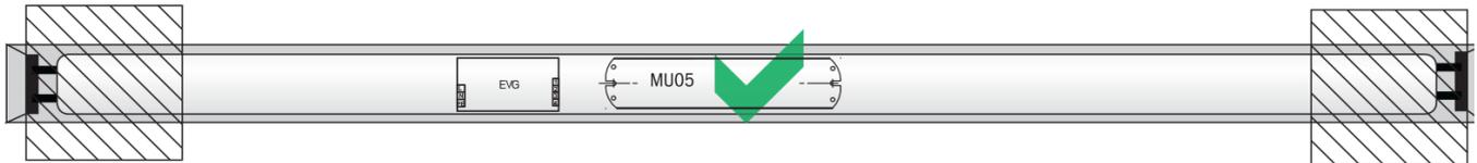
When installing the MU05 allow at least 10cm distance between the MU05 and the socket of the illuminant!
